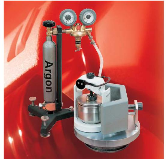
grinding in an inert atmosphere
