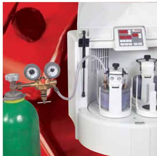
grinding in an inert atmosphere
