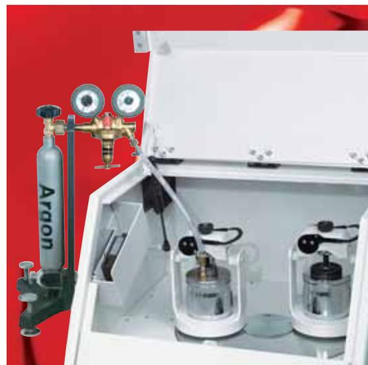
grinding in an inert atmosphere
